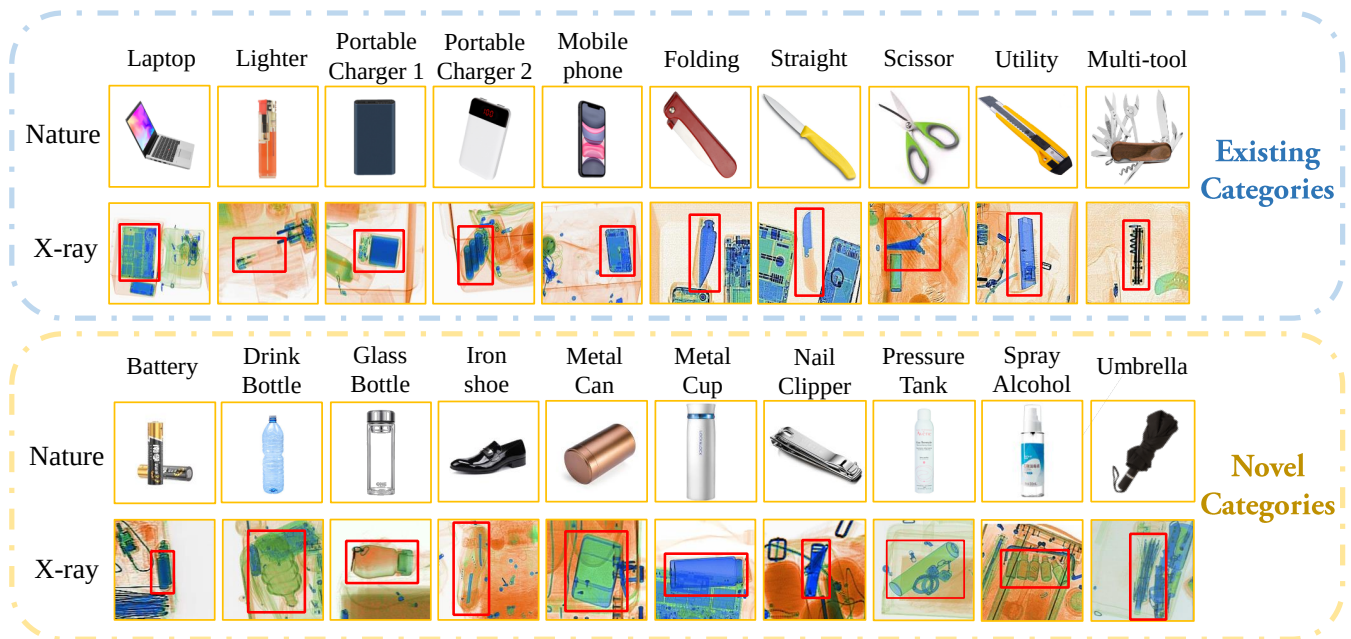
Figure 2: The X-ray images and nature images of whole 20 categories in RFS, including some common prohibited items like "Battery", "Spray Alcohol", etc.
