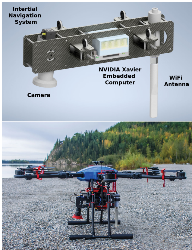
Figure 1: (Top) Rendering of the ADAPT payload assembly CAD model that is publicly available at https://kitware.github.io/adapt/ . (Bottom) Payload deployed on a sUAS.
