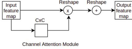
Figure 2. Details of our channel attention module
